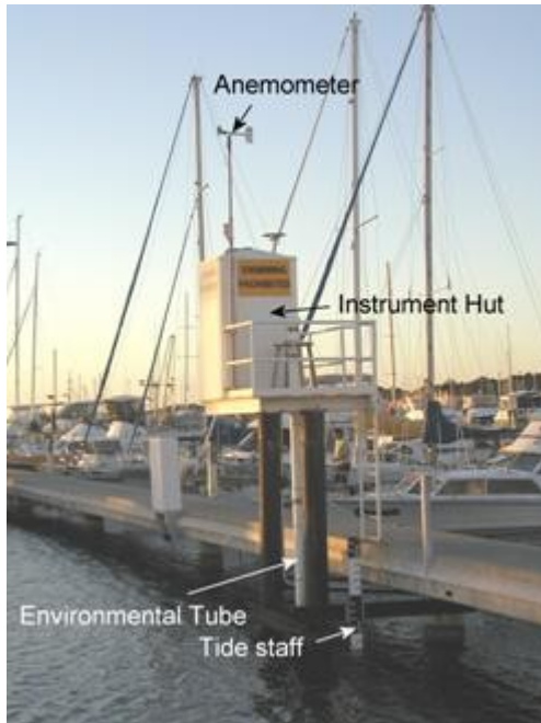
Tide gauge at Hillarys, Western Australia
